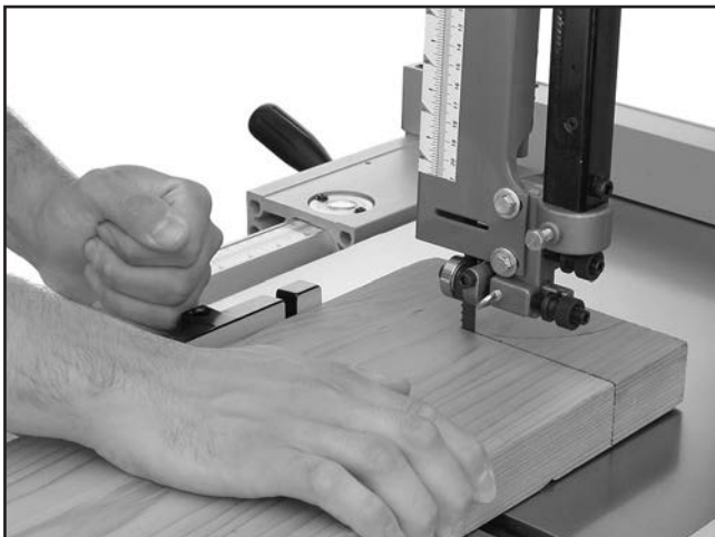
Figure 40. Crosscutting with miter gauge.
